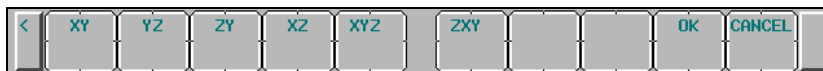
Fig. 13.2.2.2 (j) ANIMATION GRAPHIC (EXECUTION) screen (changing the graphic coordinate system) (10.4-inch LCD)
