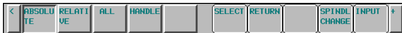
Fig. 12.4.5 (f) Soft keys displayed on the motor model code list screen (10.4-inch)
