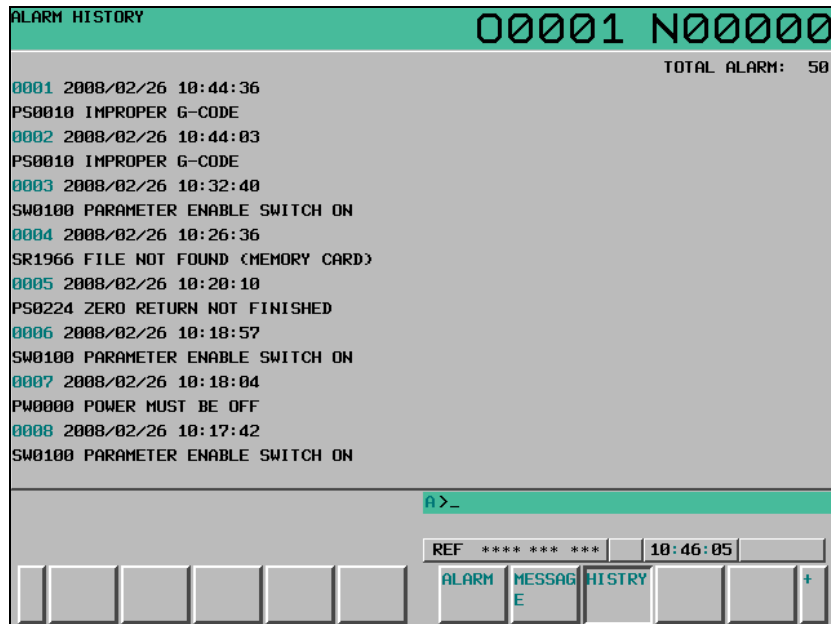
Fig. 7.2 (b) Alarm history screen (or a 2-path system, example of the 10.4-inch display unit)
